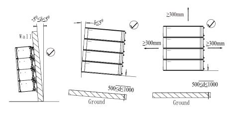
Note: The number of wall-mount installations should not exceed four.Please make sure that the weight capacity of wall should exceed 150kg.
